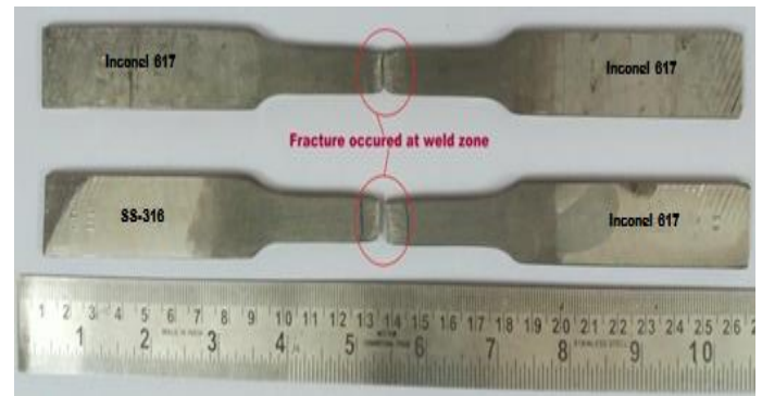
Fig- 4: Tensile test specimen after Testing
