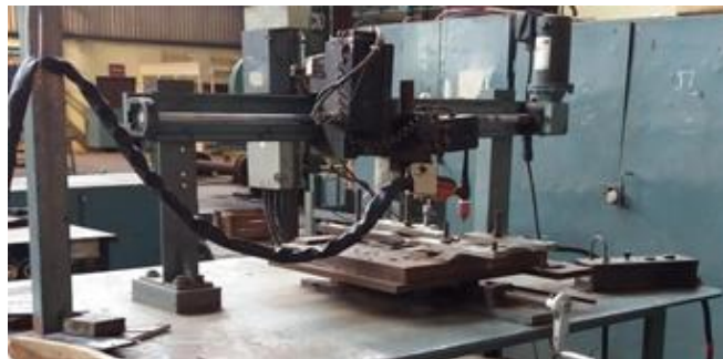
Fig-1: TIG MLS 4000 welding machine with automatic torch travel setup
