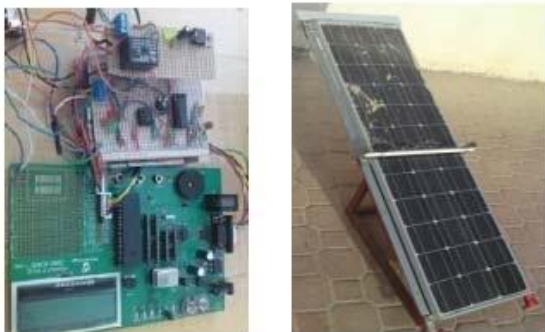
Fig. 2.12 - The cleaning process where the wiper is pulled upwards by two motors attached to the rails. It also shows the electric circuit designed to power and control the mechanical section
