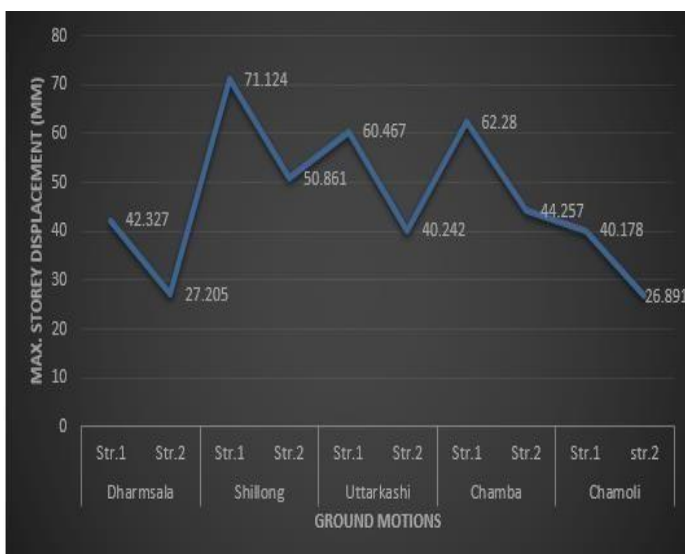
Graph 1. Maximum storey displacement(mm) vs Ground motion
