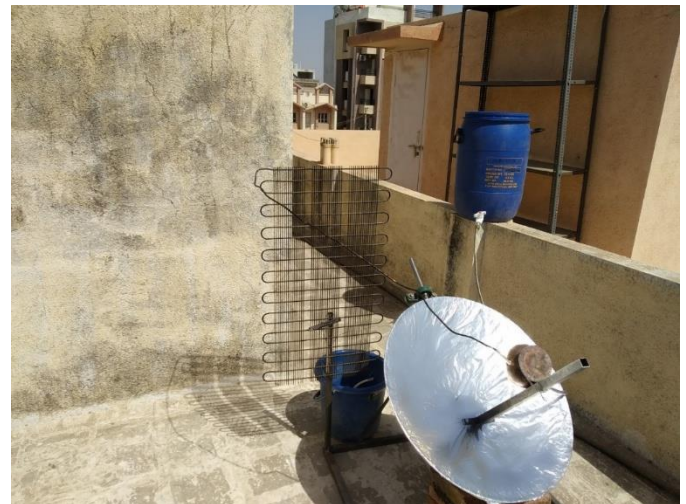
Solar concentrator of aluminium foil, without solar tracker.
