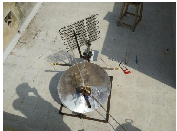
Solar concentrator of Aluminium sheet, with solar tracker.
