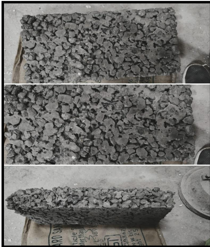
Fig. Pervious concrete sample
