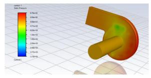
Fig -4. Pressure contour for blower M<sub>0</sub>
