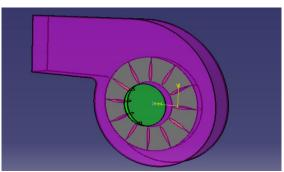
Fig -1: CATIA model of centrifugal blower
