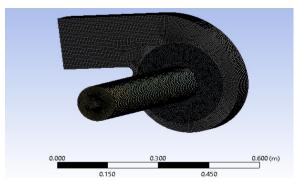
Fig -3: Meshing model of centrifugal blower
