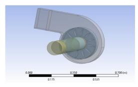
Fig -2: Centrifugal blower solid model with airfoil-curved impeller blades
