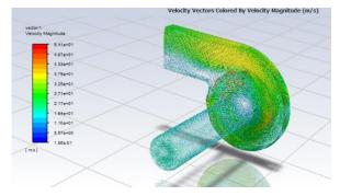
Fig -9. Velocity vector for modified blower M2
