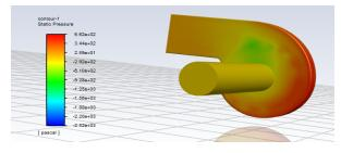
Fig -6. Pressure contour for speed M<sub>1</sub>
