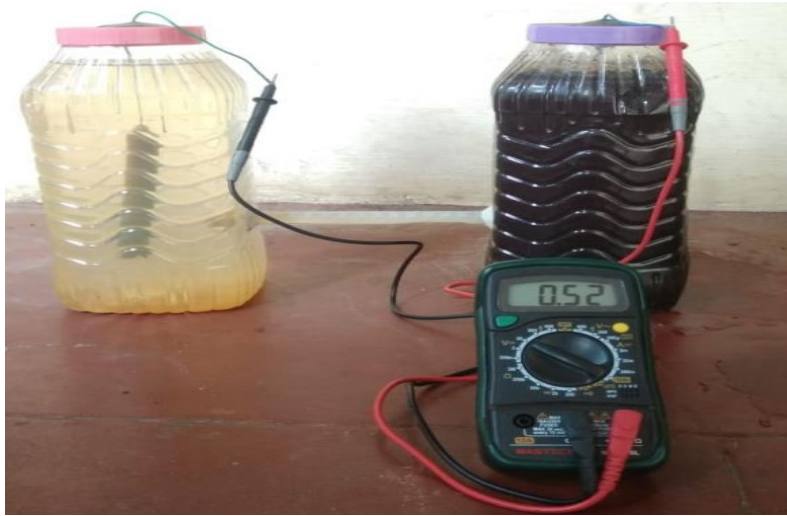
Fig 1: Double-Chambered Microbial Fuel Cell (DC-MFC) experimental setup
