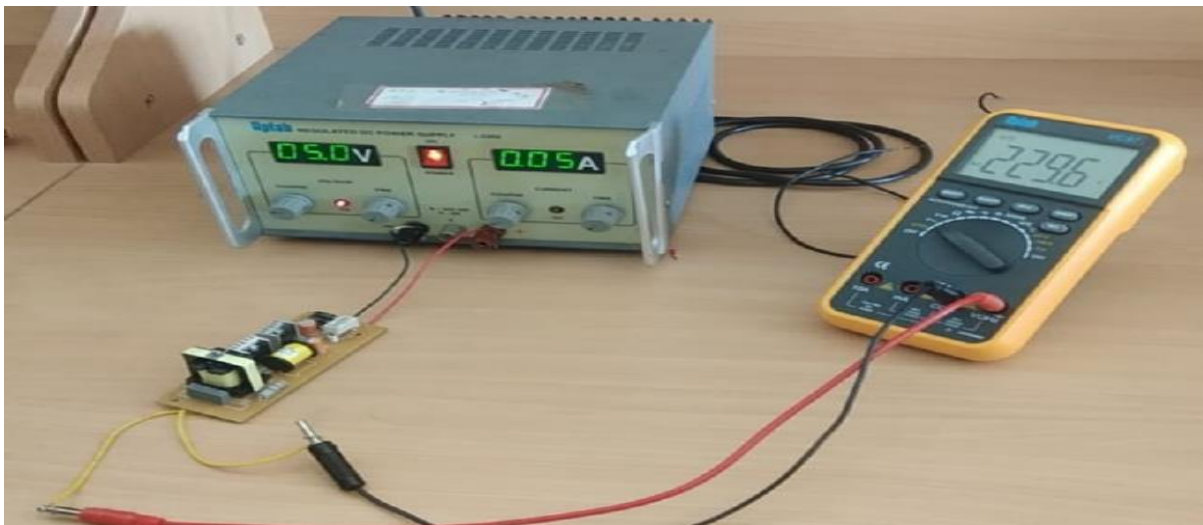
Fig 8: Output of boost converter circuit
