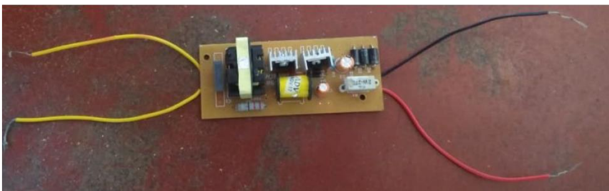
Fig 3: Proposed fabricated boost converter
