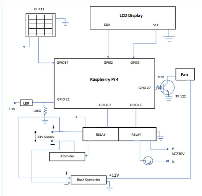
Fig 7.1: Circuit diagram
