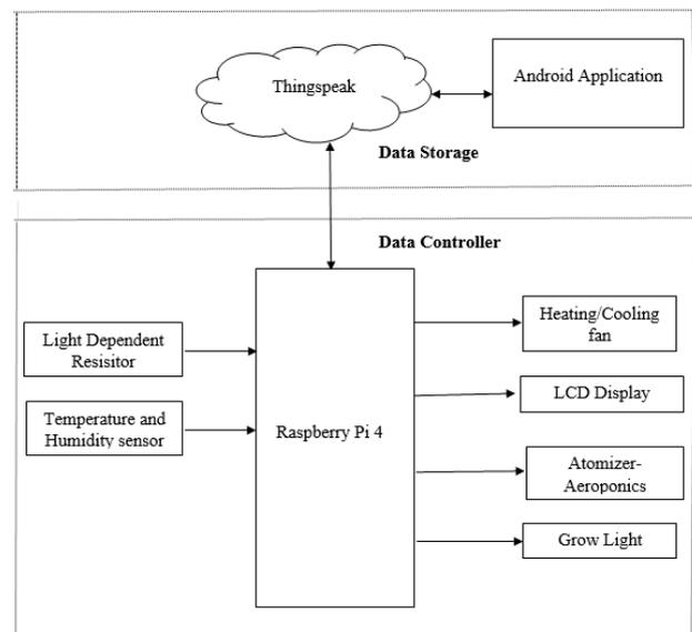
Fig.6.1 Block diagram of proposed system
