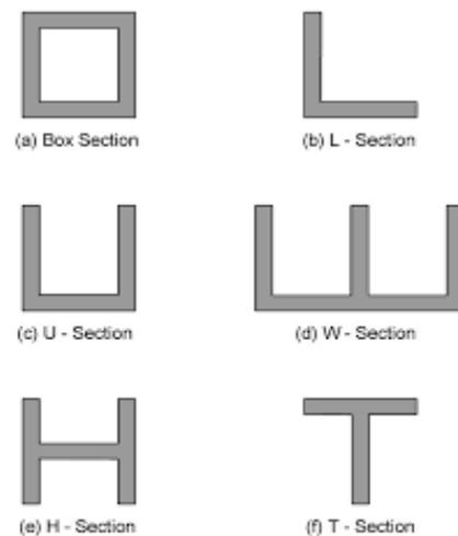
Fig. 1 Shapes shear walls.
