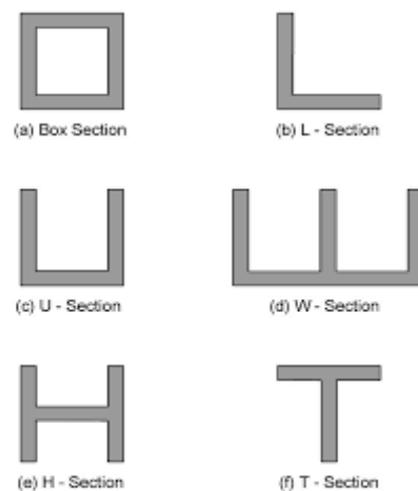
Fig. 1 Shapes shear walls.
