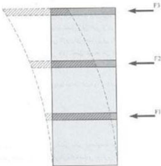
Fig. 2 Deformed shape of shear-wall under lateral load
