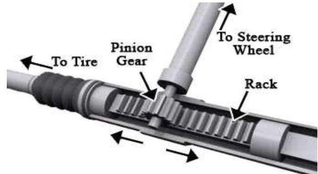
Above fig. shows the Rack and pinion steering is a simple system that directly converts the rotation of the steering wheel to straight line movement at the wheels.
