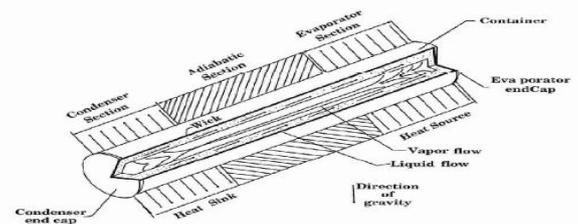
**Figure 1.1** Schematic of a conventional heat pipe showing the principle of operation and circulation of the working fluid
