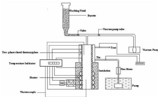
Figure 3.1 Schematic of the test rig
