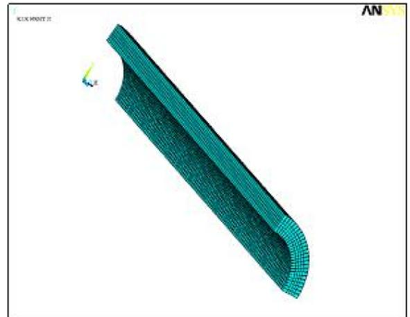
Figure-4: Mesh of the magnified model with layers
