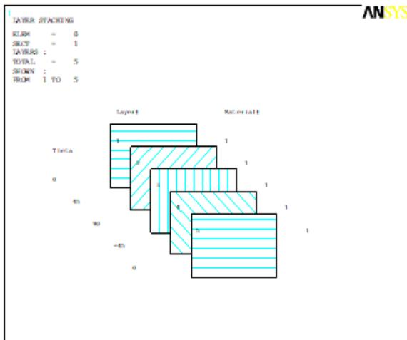
Figure-1: lay up of shell structure
