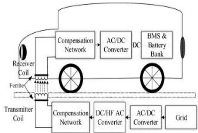
The most important thing for efficient wireless charging is to maintain the resonance frequency between transmitter coil and receiver coil so to maintain this resonant frequency compensation networks are added on both the sides. This AC power at receiver side rectified to DC through AC/DC converter and fed to the battery through Battery Management System (BMS) or Battery bank.
