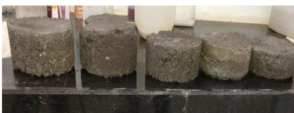
Fig 2: Concrete blocks casted using granite aggregate
