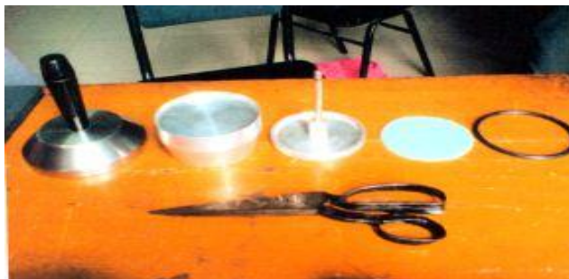
Figure 10: Accessories of Martindale Abrasion and Pilling Tester
