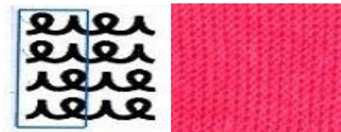
Figure 05: Chain Notation Diagram & Technical Face of Polo Pique Fabric
