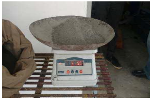
Weighing of cement and sand
