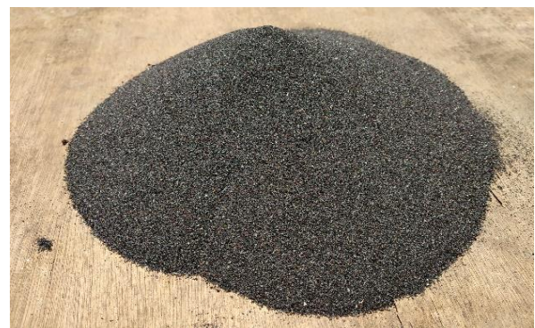
Figure 3: Used foundry sand.
