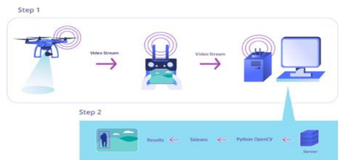
Figure 2: Architectural Diagram showing the flow of data for Real Time Object Detection on Drones
