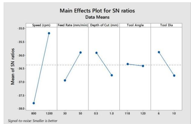
**Fig 1** Main effects plot of for S/N ratio values of Time taken
