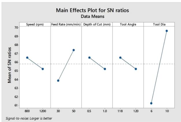
**Fig 2** Main effects plot of for S/N ratio values of MRR
