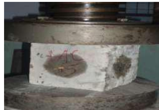
Fig -3: Compressive Strength Testing Arrangement
