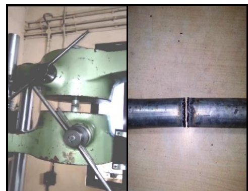
Fig 4: Tensile Test for welded Joints
