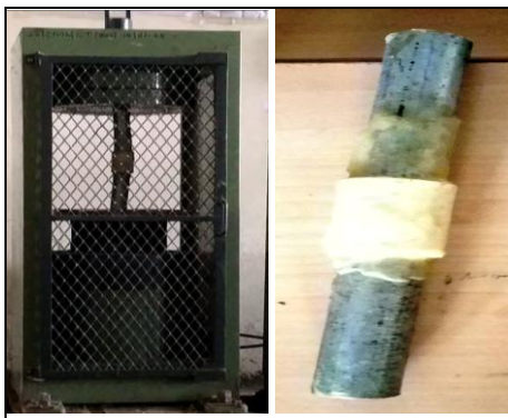
Fig 4: Compressive Test for Resin Joints
