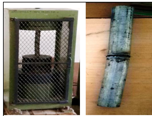
Fig 4: Compressive Test for Welded Joints
