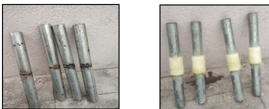
Fig 3: Welded and Resin Joint Sample
