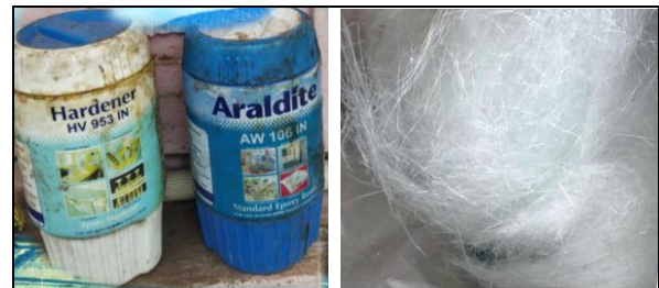
Fig -1: Epoxy Resin and Hardener & Glasswool
