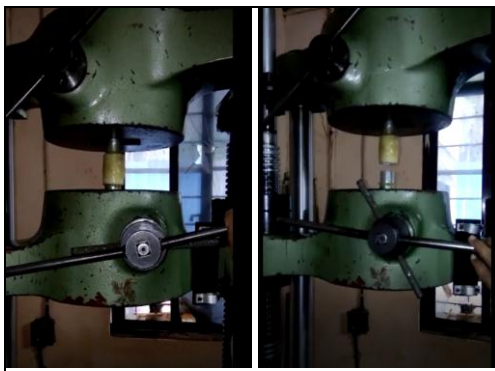
Fig 4: Tensile Test for Resin Joints
