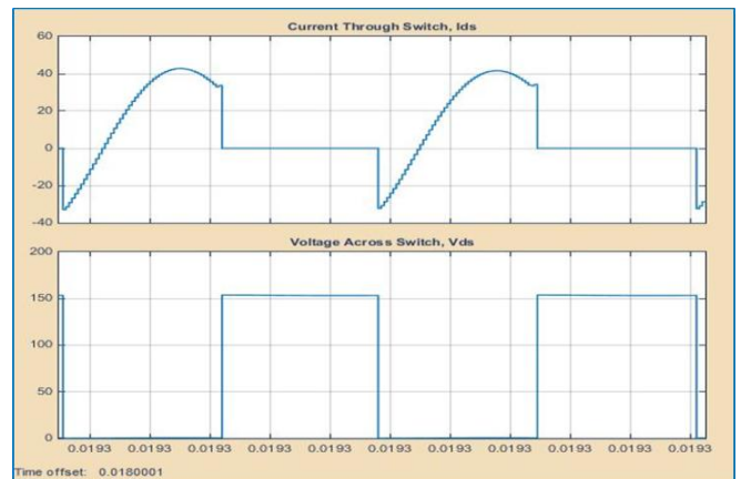
Fig.4. ZVS operation in switch
