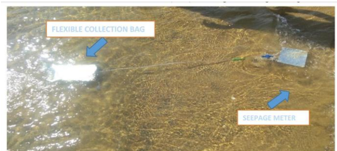
Fig -3: Seepage meter
