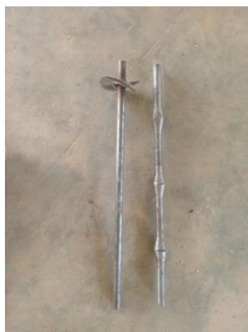
Fig -1: Helical and Waveform pile
