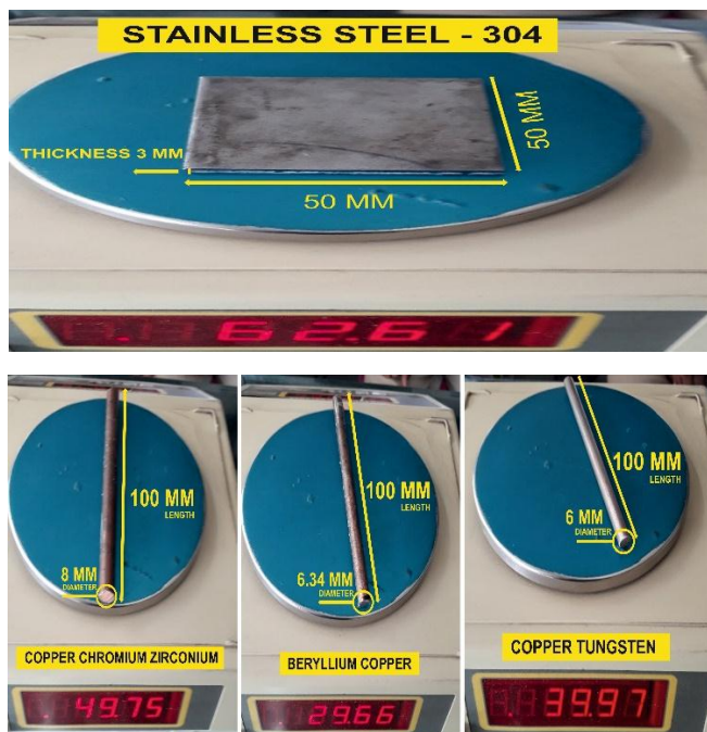
Fig.2 Work Piece and Electrode Material
