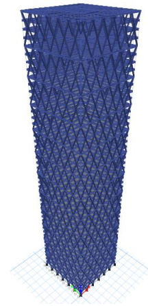
Fig -12: Elevation view of Model-1 with diagrid angle D4
