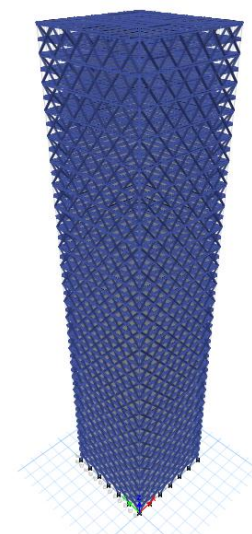
Fig -8: Elevation view of Model-1 with diagrid angle D2
