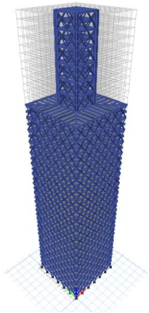
Fig -9: Elevation view of Model-2 with diagrid angle D2
