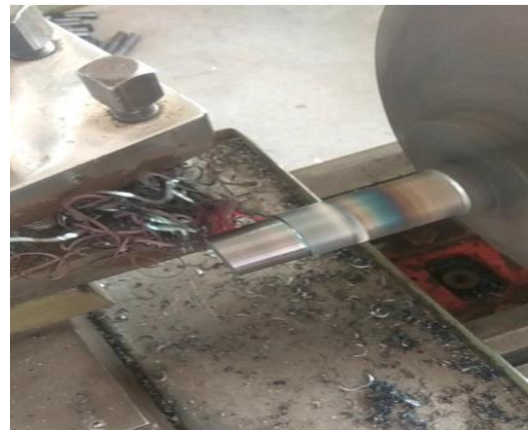
Chip Formation of Hot Machining
