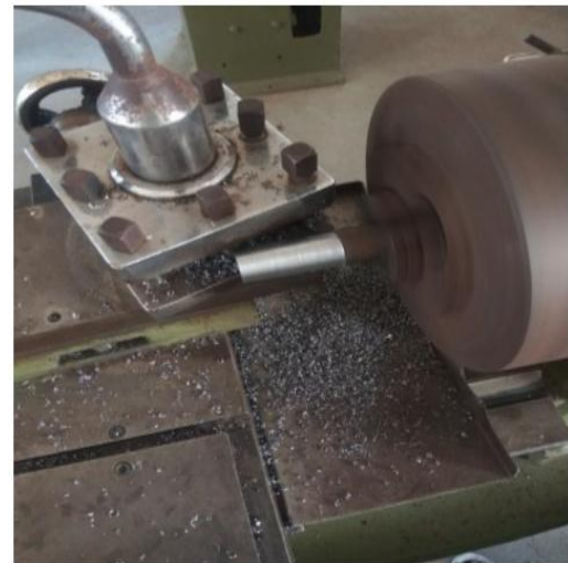
Chip Formation of Normal Machining
