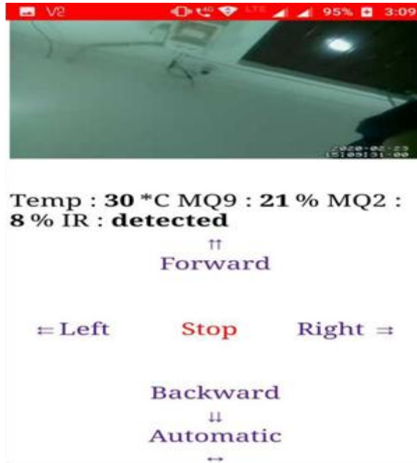
Fig3: IOT page displaying the presence of obstacle through IR sensor
