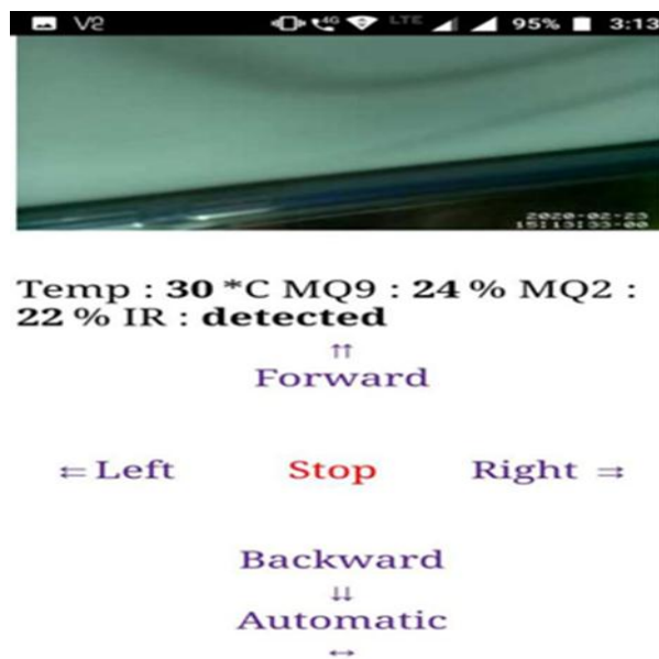
Fig4: IOT page displaying an increase in gas levels (MQ2 and MQ9)
