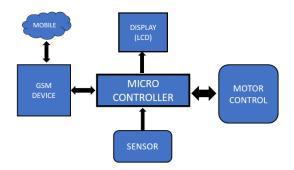
In the normal vehicle, we need ignition key to turn on or off the system, but in this electric motorcycle we can start or stop by mobile application through the GSM device. Where the accident is detected by microcontroller using vibration sensor in the motorcycle and the location is sent to the mobile number which is fed to the system.
