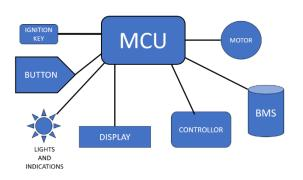
The electric motorcycle as two riding modes of economy mode and sports mode. In the eco mode the EV runs at low speed and gives high range, in sports mode the EV runs at high speed and gives low range. This mode change data is transfer to the motor drive controller from the microcontroller. The state of the mode is shown on the LCD display.
