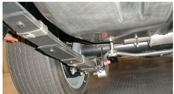
Figure - 1.1: A traditional leaf spring arrangement.
