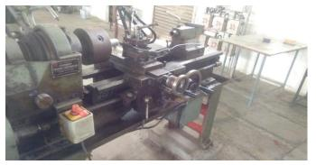
Fig.2.1 Centre lathe machine
