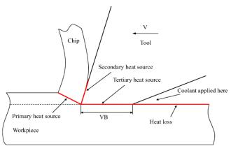
Fig.1.1 Sources of heat generation in orthogonal cutting process.
