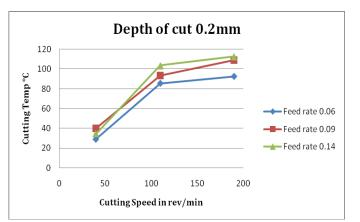
Fig 3. 1 Temperature v/s cutting speed at varying feed rate on depth of cut = 0.2mm
