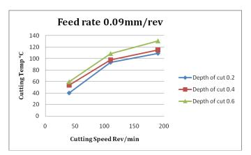
Fig 3. 5 Temperature v/s cutting speed at varying Depth of cut on Feed rate = 0.09mm/rev
