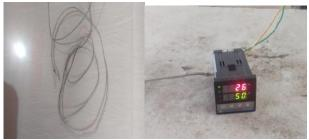
**Fig.2.2** (a) Thermocouple (b) digital temperature indicator
