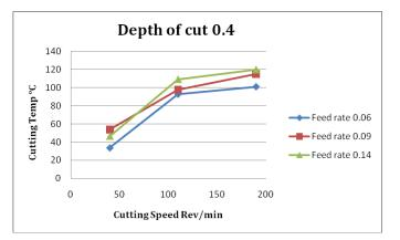
Fig 3. 2 Temperature v/s cutting speed at varying feed rate on depth of cut = 0.4mm
