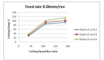
Fig 3. 4 Temperature v/s cutting speed at varying Depth of cut on Feed rate = 0.06mm/rev
