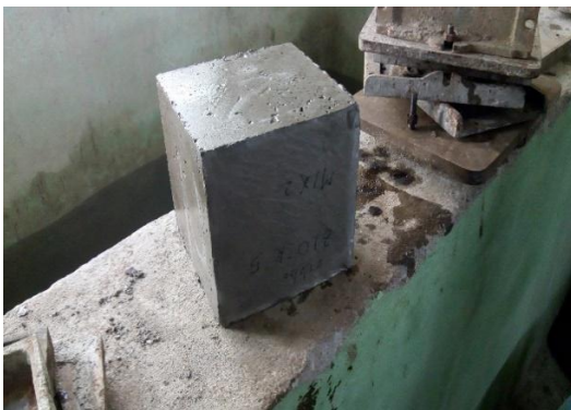
Fig -1: Concrete block after 28 days curing
