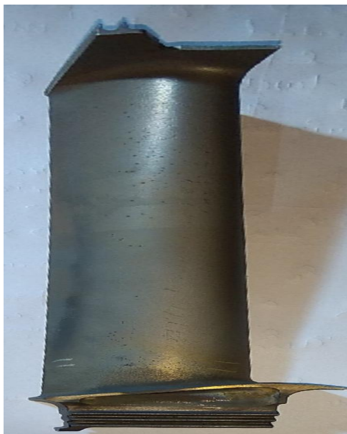
Fig -2: LP Turbine blade
