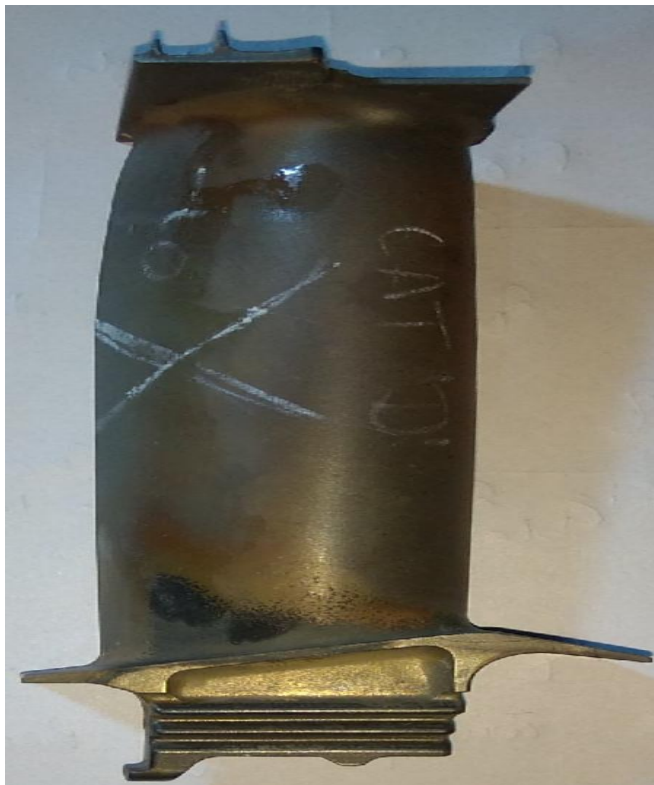
Fig -1: HP Turbine blade
