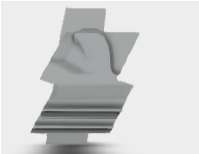
Fig -5: Front view of HP blade
