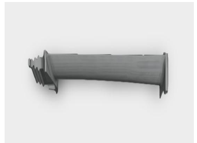
Fig -10: Top view of LP blade
