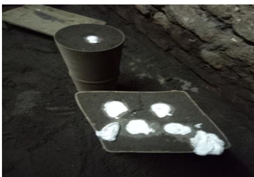
Figure 2: Die pattern & casting product
