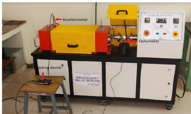
Fig -4: Experimental Setup of Gearbox Test Rig
