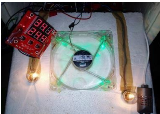
FIG 20: Bulbs are on when temperature is below 36°C
