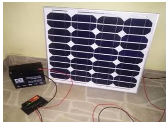
FIG 7: PV system components connections
