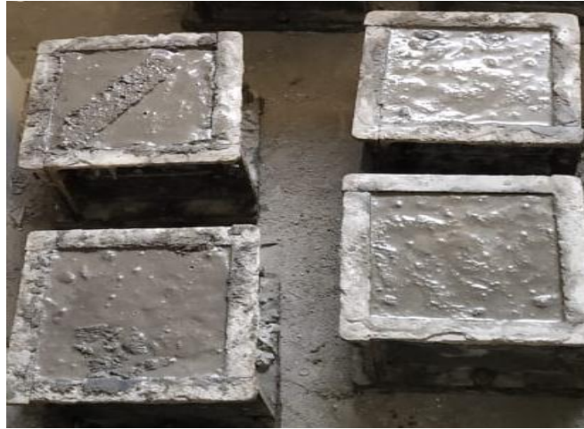
Fig.2 Casting of cubes
