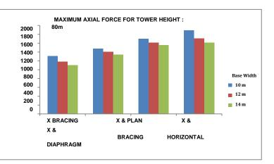
**Chart: 3** Comparison of Maximum Axial Force for Tower Height: 80m
