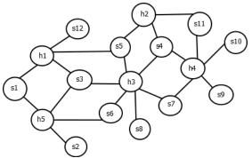
Fig .WSN with sensor nodes and head nodes
