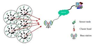
Fig2: Cluster based WSN model. 1.1.2 Wireless Sensor Network requirements
