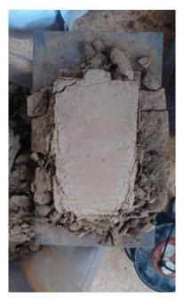
Figure -4: Specimen of crushed interlocking blocks form compression test
