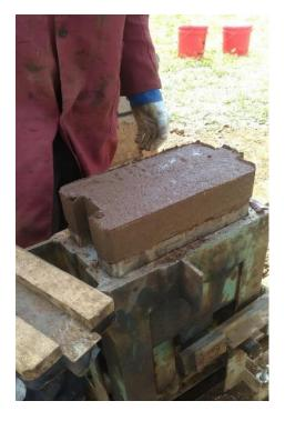
Figure -2: Interlocking block on Block Press Equipment
