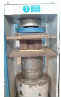
Figure -3: Interlocking block specimen placed on the compressive test machine
