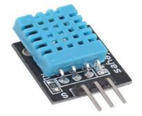
Working principle of DHT11 Sensor:
