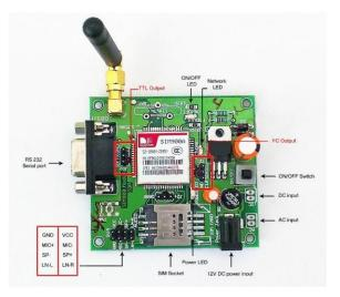
In GSM Modem we are going to use only four pins.
