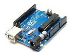
The Arduino Uno is a microcontroller board based on the ATmega328. It has 14 digital input/output pins (of which 6 can be used as PWM outputs), 6 analog inputs, a 16 MHz ceramic resonator, a USB connection, a power jack, an ICSP header, and a reset button. It contains everything needed to support the microcontroller; simply connect it to a computer with a USB cable or power it with a AC-to-DC adapter or battery to get started.
