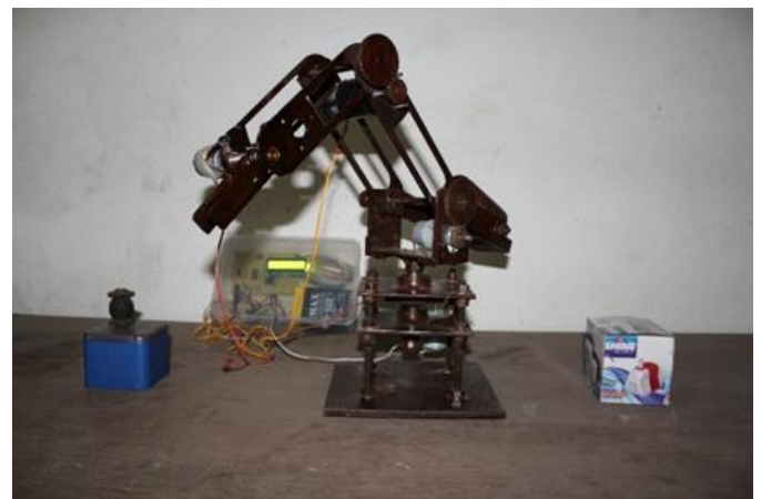
Fig -6: Manufactured assembly of robot manipulator
