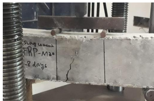
Fig 4 Flexural Strength Test
