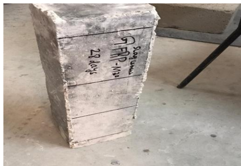
Fig 3 Marking for Flexural Strength Test
