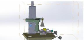
Fig-8: High-performance laser distance sensors position
