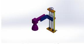
Fig-3:. Laser Mount Column
