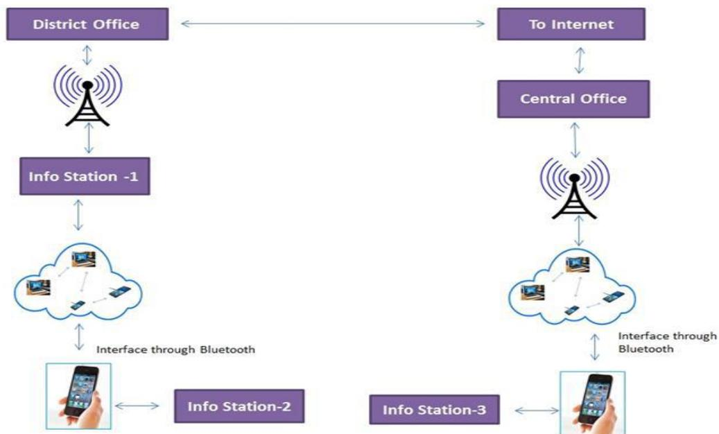
**Fig.3**Proposed Architecture of Remote Data Acquisition system
