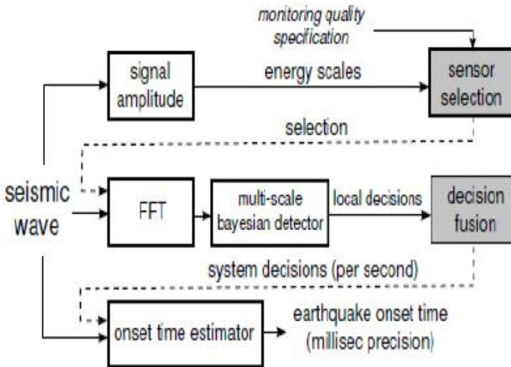
**Fig.2** Architecture for Detection of Earthquake
