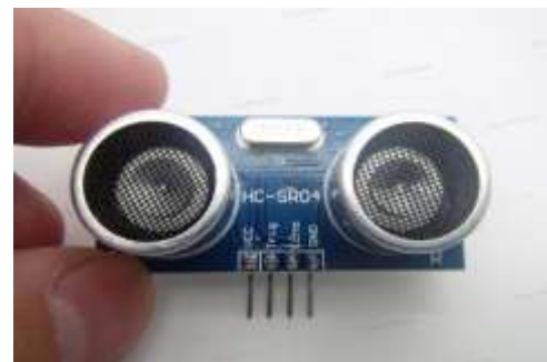
Fig -3: Pin Diagram of HC-SR04 ultrasonic sensor
