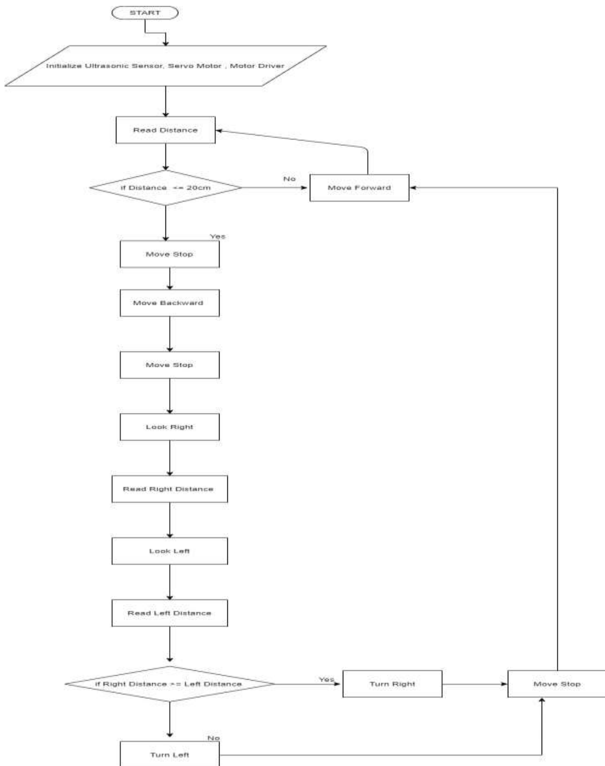
Fig -5: System Work-flow
