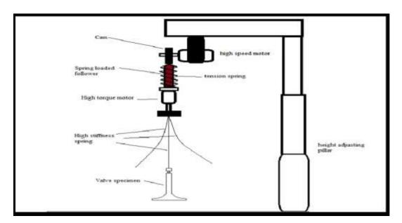
Fig.1 Diagram of Valve Lapping Machine
