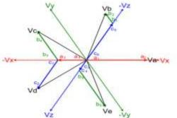
Phasor diagram of the proposed transformer connection (star-star).
