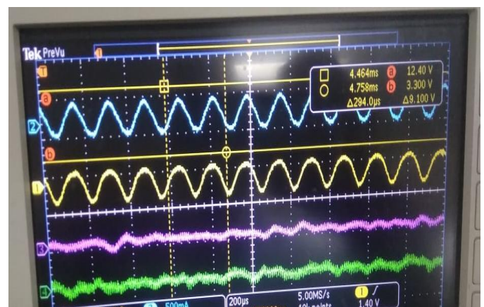
Fig 5: Ripple voltage for 90V input
