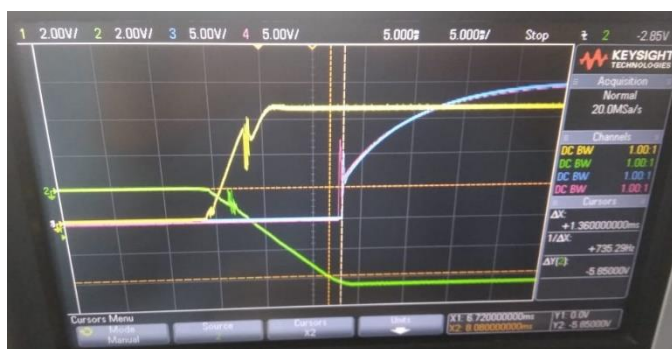
Fig 8: Output voltage of both the outputs during start-up
