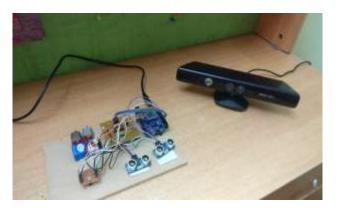
Fig -4: Assembled module with KINECT sensor
